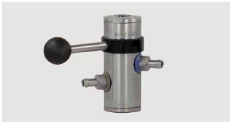
1/2" F : 1/2" F. Injector ST-168 with hose tail 9 mm and compressed air module (hose tail 9 mm). The chemical dosing is adjusted by 10 exchangeable nozzle inserts (0.5 - 2.0 mm). Max. 350 bar / 100 °C
