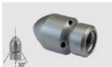
3/8" F. Outside \varnothing 30 mm. 4 rear jets, with front jet
