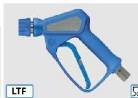
Pro gun with patented LTF technology and progressive closing system. Gun with coupling ST-3100. Field of application: foam and rinsing applications in the food industry etc. Stainless steel. Chemically resistant valve piston stainless steel. PEEK piston. Max. 80 bar / 80 l/min / 150 °C
