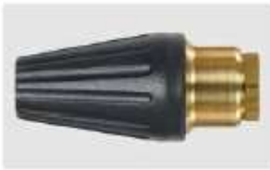
1/4" F. Spray angle 20°. 120 - 250 bar. Max. 100 °C Kit ST-458.1
