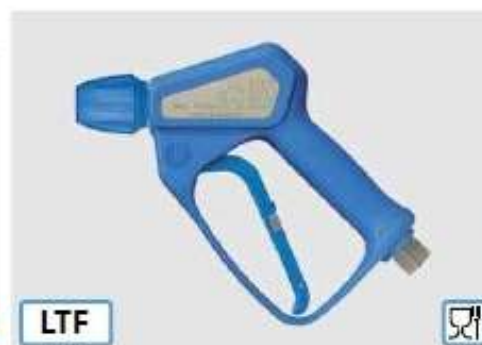
Professional gun with patented LTF technology. Stainless steel. Gun with coupling KW. Max. 310 bar / 45 l/min / 150 °C
