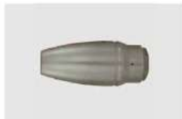
1/4" F. Spray angle 20°. Max. 700 bar / 90 °C. Delivery time of approx. 1 week
