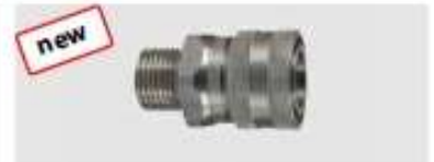
Coupling : M. Stainless steel. 60° cone. Max. 250 bar / 150 °C
