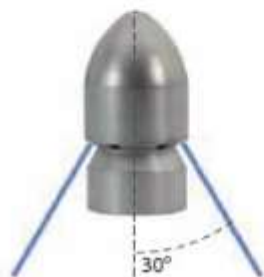
1/4" F. Outside \varnothing 25 mm. 6 rear jets, with front jet
