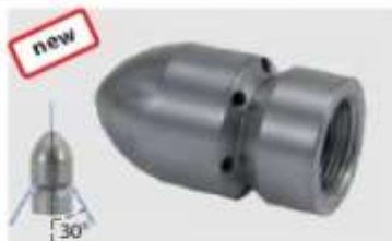
3/4" F. Outside \varnothing 38 mm. 6 rear jets, with front jet
